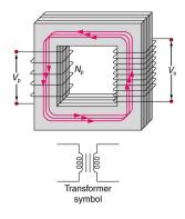
For a simple transformer such as the one shown above, the output voltage depends almost entirely on the input voltage and the ratio of the number of loops in the primary and secondary coils. Faraday's law of induction for the secondary coil gives its induced output voltage to be:
