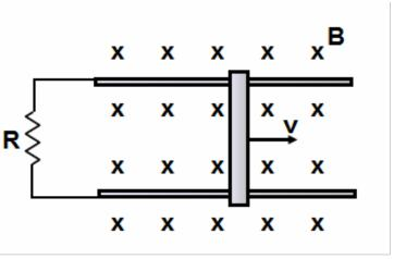
f. Determine the power dissipated in the resistor when the rod crosses the magnetic field.
